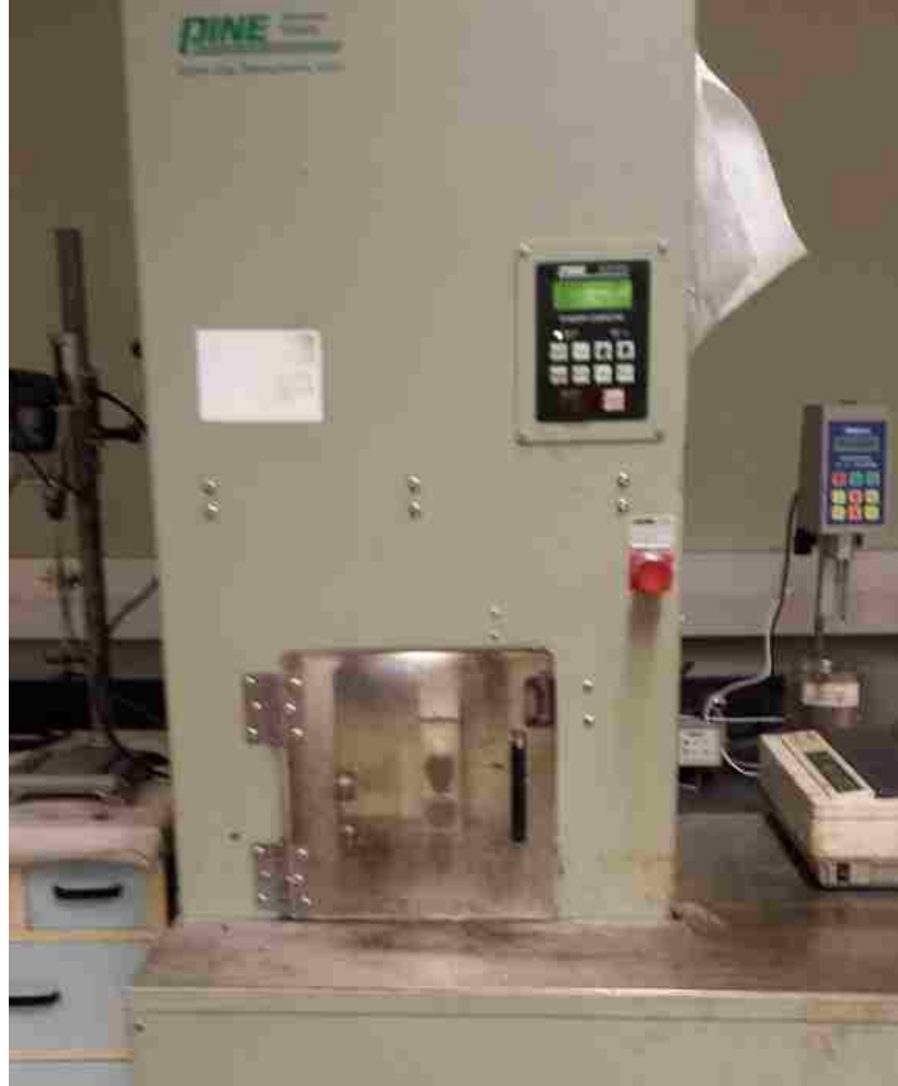
Figure 3.4: Pine Gyrotory Compactor
