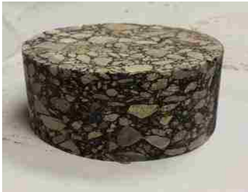
Figure 3.19: IDT Asphalt Concrete Sample
