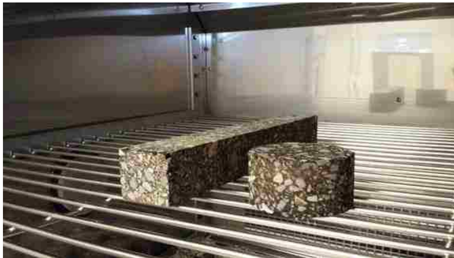
Figure 3.14: Samples Being Conditioned by Freeze-Thaw Method
