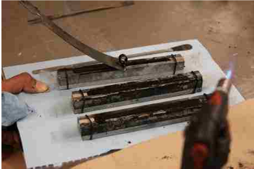
Figure 3.6: Trimming of Room Temperature Binder Sample
