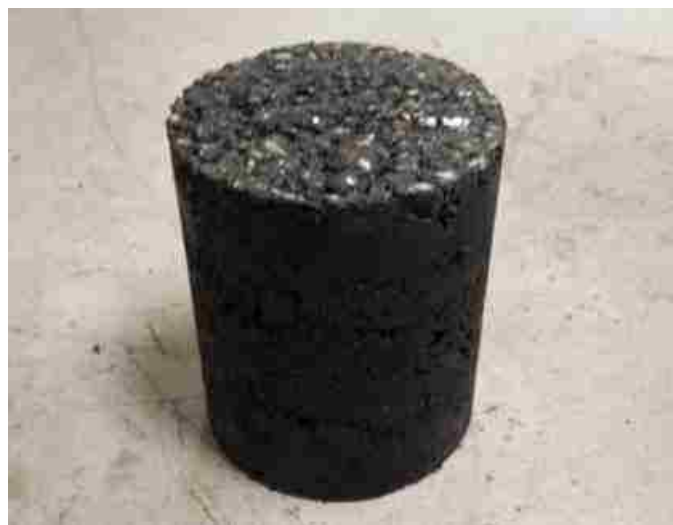
Figure 3.5: Molded Sample with 8 inches Height and 6 inches Diameter
