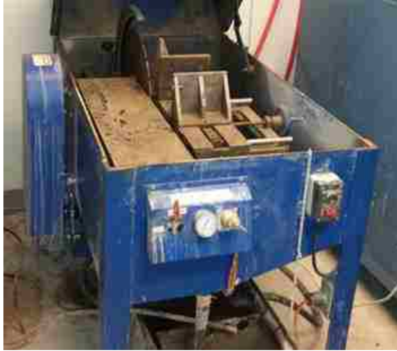
Figure 3.10: GCTS stone-cutting saw with original clamps
