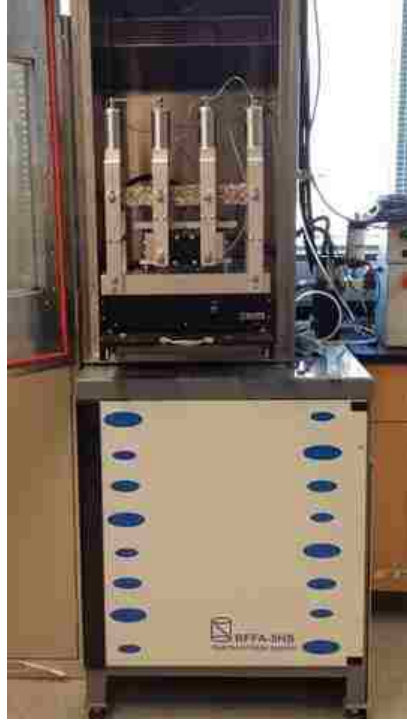
Figure 3.16: GCTS Flexural Beam Setup
