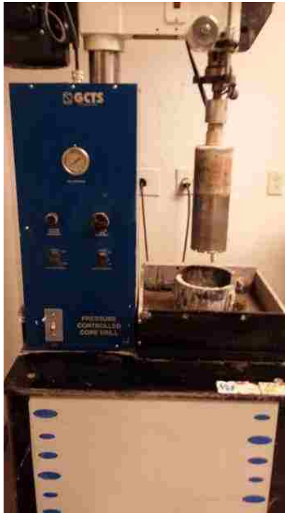
Figure 3.12: GCTS Pressure Controlled Core Drill
