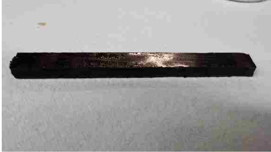
Figure 3.7: Finished BBR sample
