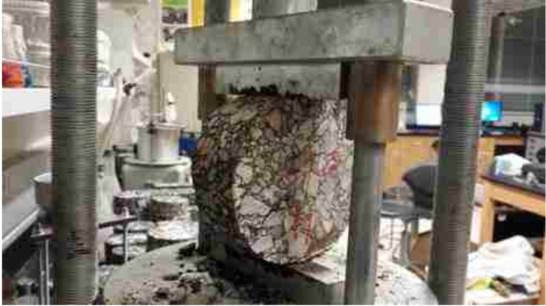
Figure 3.20: IDT Test Setup with a Specimen
