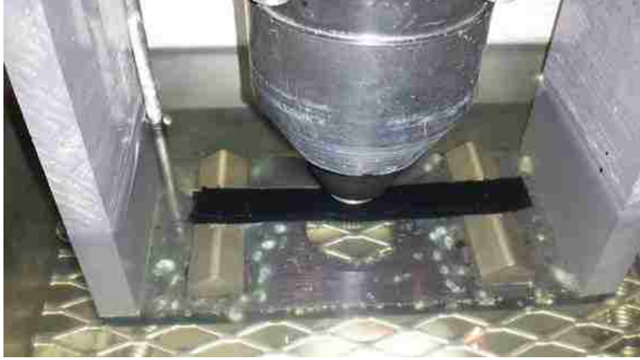
Figure 3.23: BBR Test Setup with a Sample
