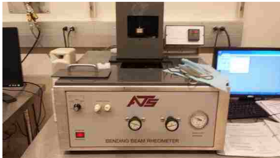
Figure 3.22: BBR Testing Apparatus
