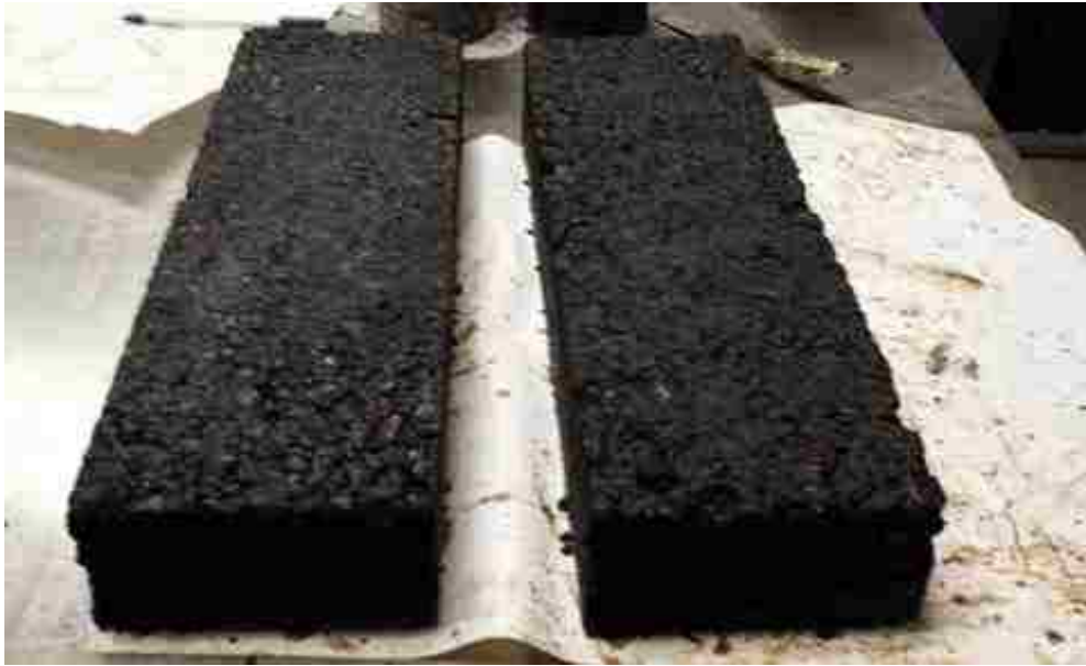
Figure 3.9: Uncut Hot Mix Asphalt Beam Samples
