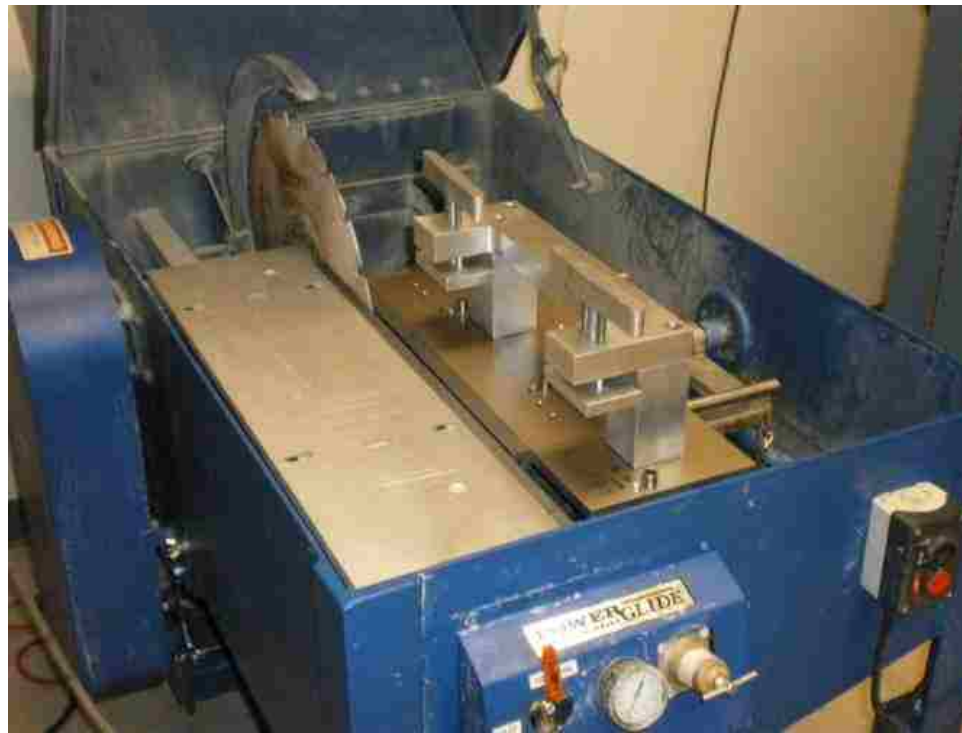
Figure 3.11: GCTS stone-cutting saw with modified clamps
